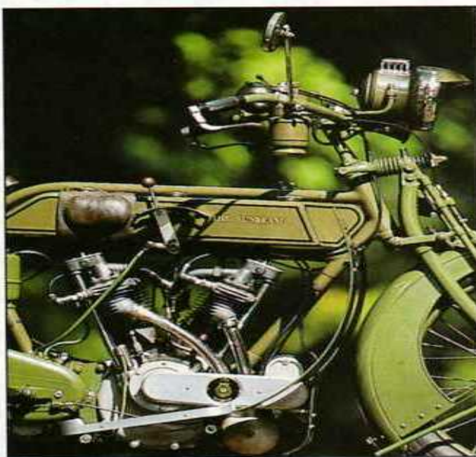
Tank has three sections; oil at the front, petrol at the rear, and the largest compartment, for paraffin, in the middle. Overhead inlet valve mechanism of the 992cc MAG engine is fully enclosed.
