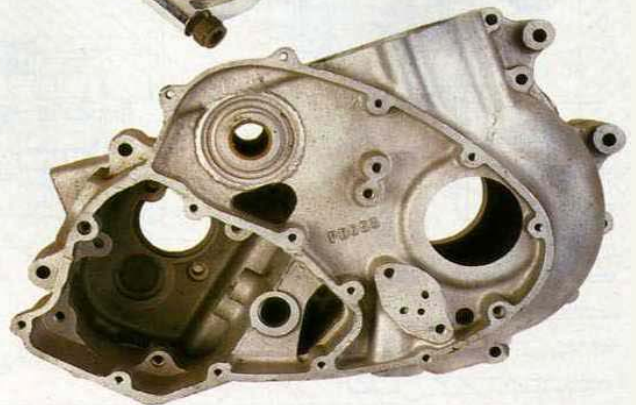
Below: crankcase/gearbox castings: single camshaft's bushes are in upper portion
